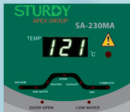
C. Progress indicator
